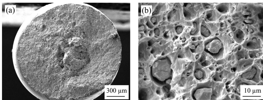
**Fig.4 Fracture appearances of Ag-10% $\text{SnO}_2$  material**
