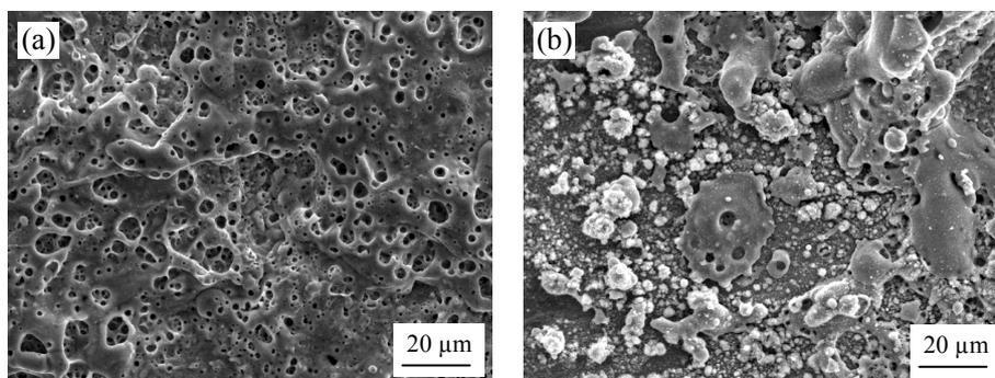
**Fig.5 Arc erosion surface of  $\text{AgSnO}_2$  material for anode (a) and cathode(b)**
