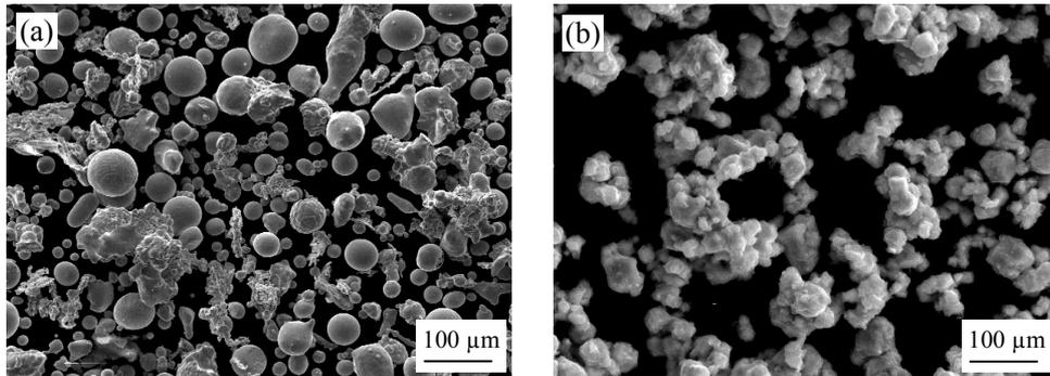
Fig.1 SEM images of the raw powders for Ag (a) and SnO<sub>2</sub> (b)
