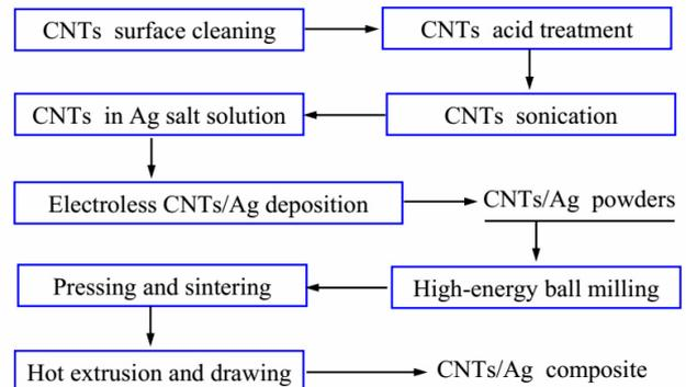
Fig.1 Schematic fabrication process for chemical plating preparations of CNTs/Ag composite
