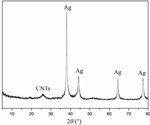
Fig.3 XRD patterns for CNTs/Ag composite powders
