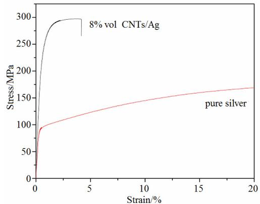
Fig.7 Stress-strain curves of CNTs/Ag composite and pure Ag
