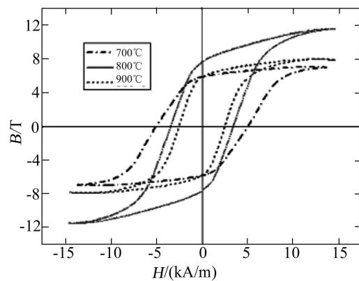
Fig.4 Hysteresis loops of the SPS Fe<sub>50</sub>Pt<sub>50</sub> alloy sintering at different temperatures
