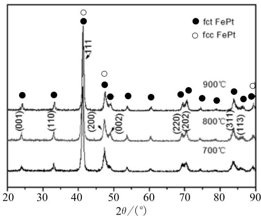
Fig.2 XRD patterns of FePt alloys processed by spark plasma sintering
