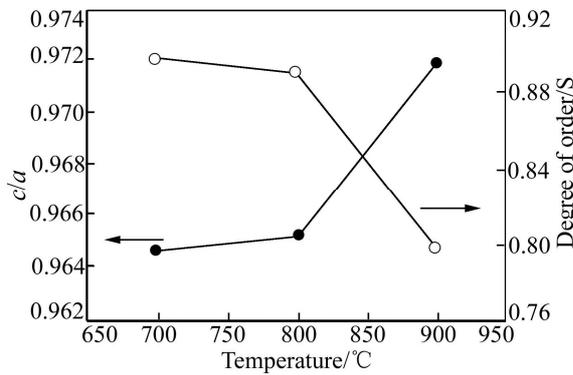
Fig.3 Axial ratio  $c/a$  and degree of order of  $Fe_{50}Pt_{50}$  alloys SPSed at different temperatures
