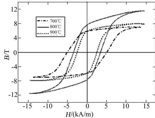
Fig.4 Hysteresis loops of the SPS  $Fe_{50}Pt_{50}$  alloy sintering at different temperatures
