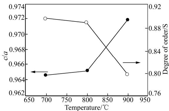
Fig.3 Axial ratio c/a and degree of order of Fe<sub>50</sub>Pt<sub>50</sub> alloys SPSed at different temperatures
