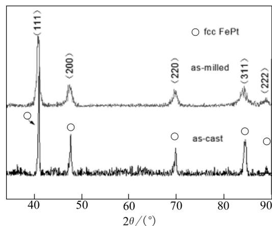
Fig.1 XRD patterns of FePt alloy on as cast and as milled samples
